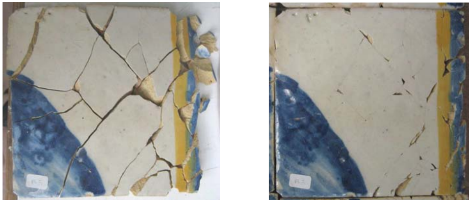
Figure 1. Tile fragments re-adhesion. A) Fragmented tile and b) Tile after fragment re-adhesion treatment. Images by Maria de Lurdes Esteves.
